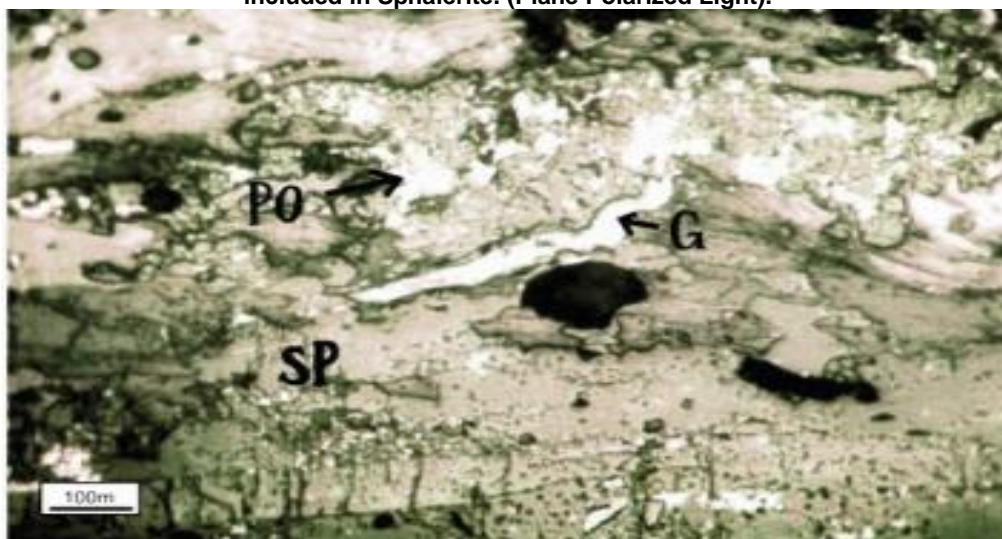
Fig. 11: A graphite (G) Grain is being kinked within Sphalerite (SP) Matrix. Pyrrhotite (PO) Grains are included in Sphalerite. (Plane Polarized Light).
