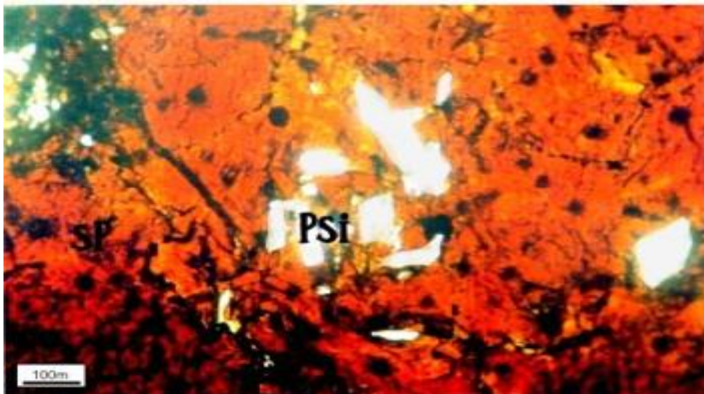
Fig. 8: Elongated Pyrrhotite (Po) Grains Are Oriented within the Sphalerite (Sp) Matrix. (Plane Polarized Light).
