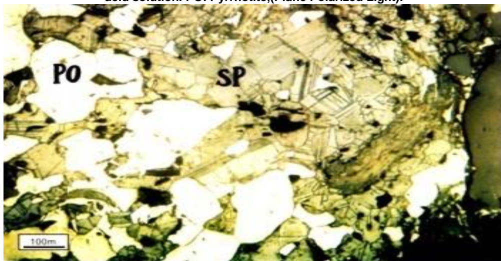
Fig. 11: A graphite (G) Grain is being kinked within Sphalerite (SP) Matrix. Pyrrhotite (PO) Grains are included in Sphalerite. (Plane Polarized Light).
