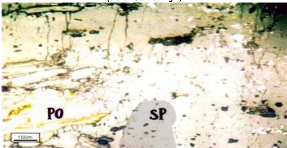
Fig. 8: Elongated Pyrrhotite (Po) Grains Are Oriented within the Sphalerite (Sp) Matrix. (Plane Polarized Light).
