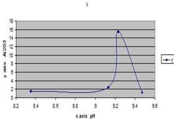
Observation of Alumina Percentage (Al<sub>2</sub>O<sub>3</sub>) for 0.3 g carbon source for 34% ore
