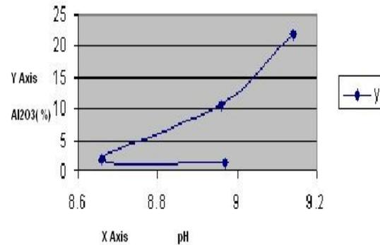
pH progressively increased during bioleaching due to alumina solubility and reached a maximum of 9.47 in case of 0.3g carbon source where alumina % being 15.50 after 15 days of incubation and then decreased. Such an effect can be justified that increasing in pH results in the ability of metabolite to dissolve alumina. Thus after 20 days there was no complexation reaction occurred between alumina and organic acids released by the microorganisms.
