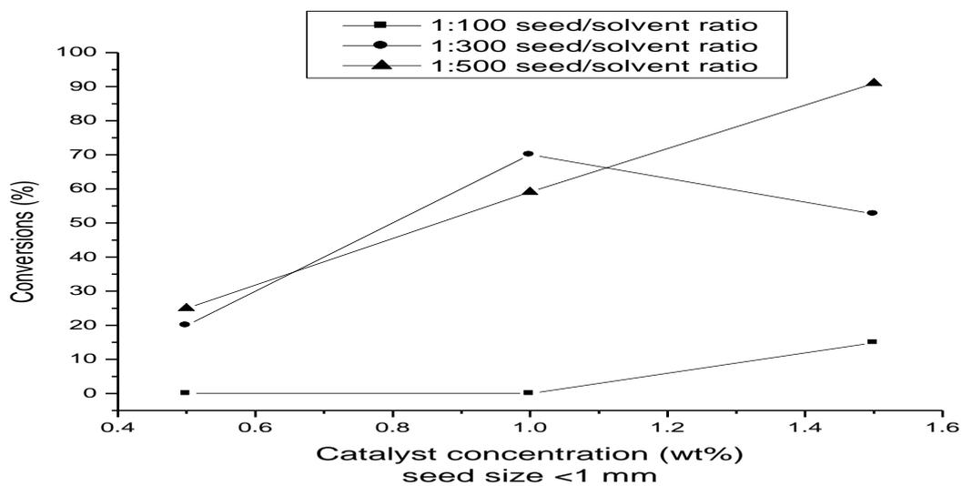
Fig 4: The effect of Catalyst Concentration (Wt %) and Seed / Solvent Ratio of Biodiesel Conversion on Seed Size >1-<2 mm.
