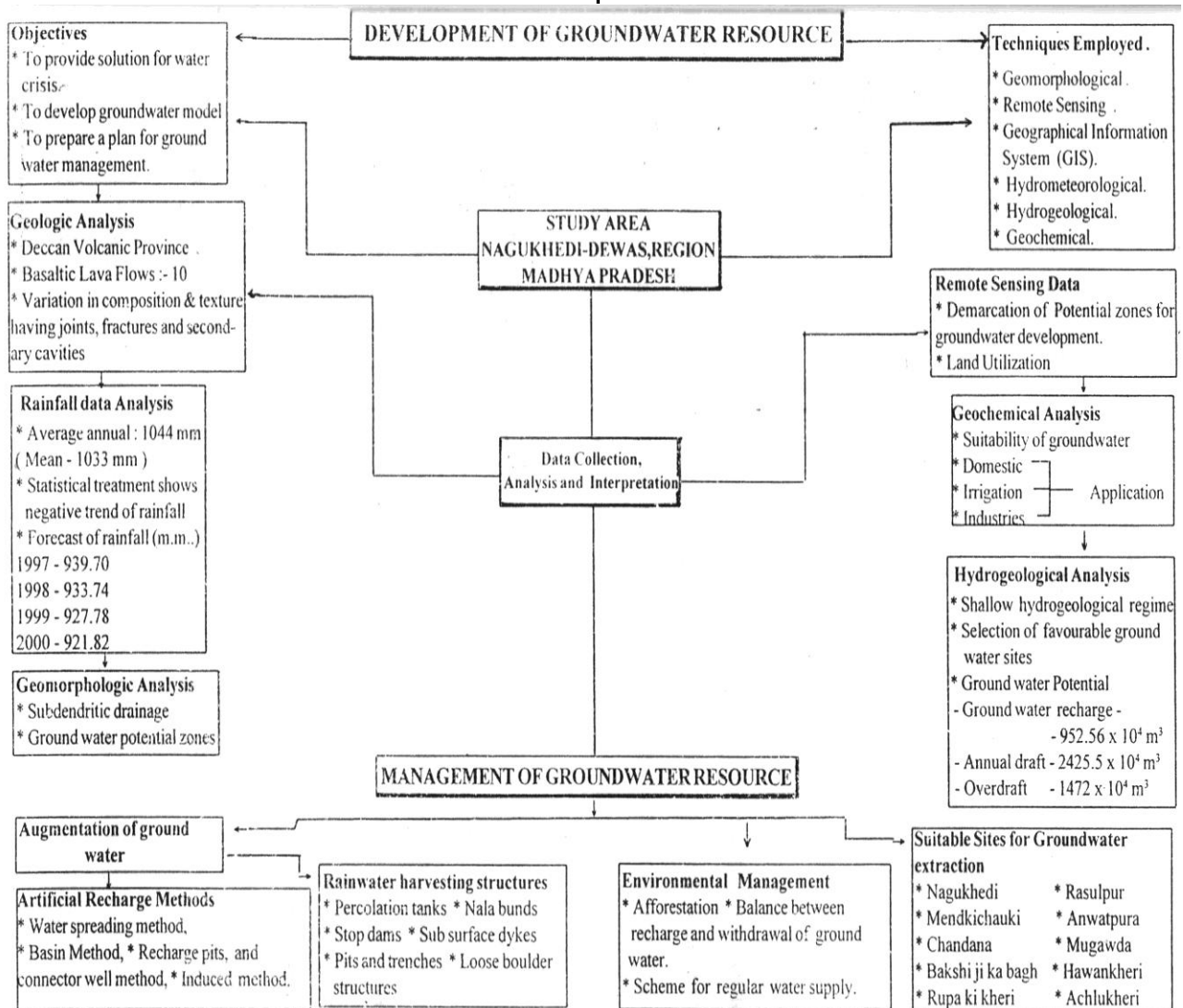
Figure 4 Groundwater Model of Nagukhedi – Dewas Area, M.P. based on Integrated Remote Sensing Technique
